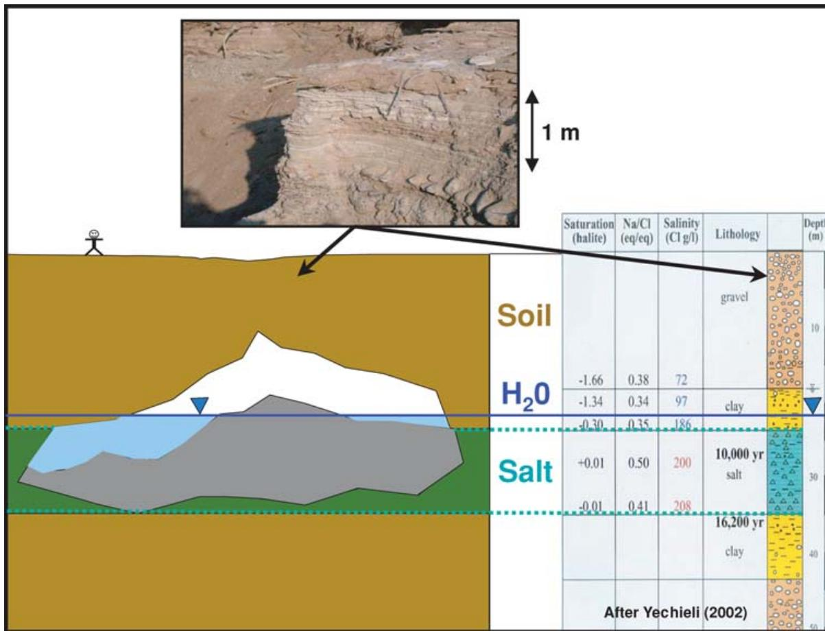
**Figure 2.** Schematic diagram of a sinkhole and mature cavity in the subsurface according to local borehole log (Yechieli 2002) with detailed photograph of the layered media. Groundwater depth is below 20 m and salt is found between 23 and 35 m depth.
