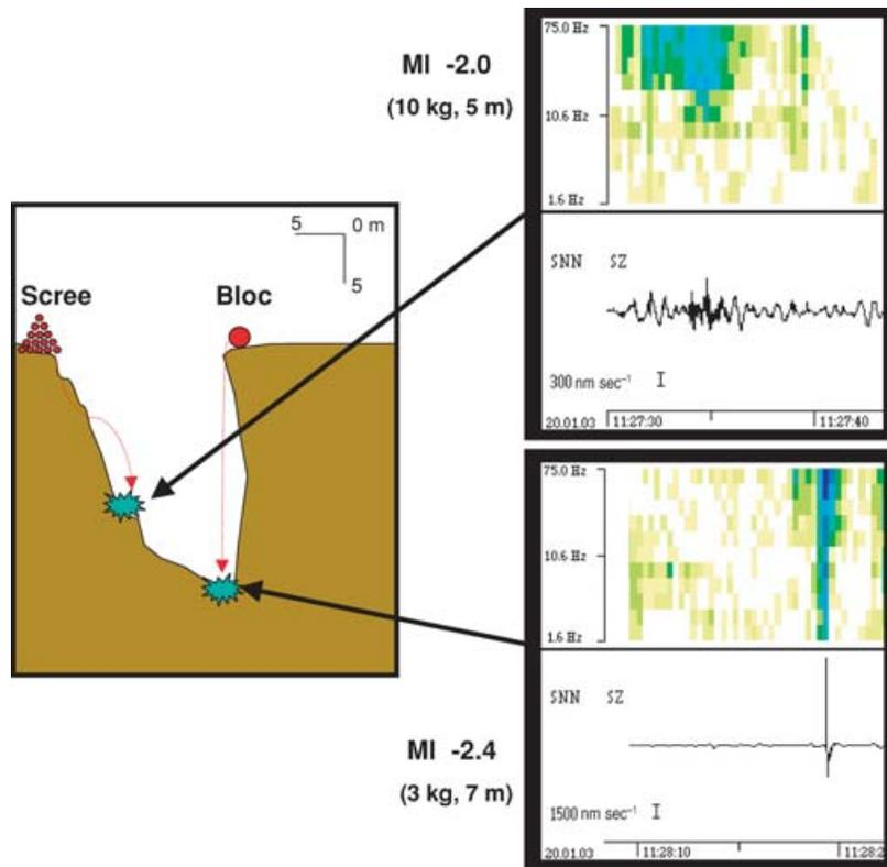
**Figure 6.** Source signal simulation in the field: Waveforms and sonograms generated by impacts in an open dry sinkhole by a rock-debris fall (top) and by a single bloc (bottom).
