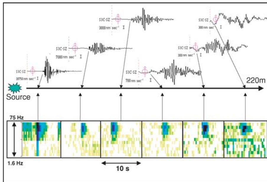
**Figure 8.** Stability of the sonogram analysis for source-to-sensor distances from 20 to 220 m. Sonograms display the vertical component in constant 10 s time windows. Corresponding waveforms with varying amplitudes (see scale bars) and constant 3 s window are displayed for comparison. The signal source is an impact at the surface.
