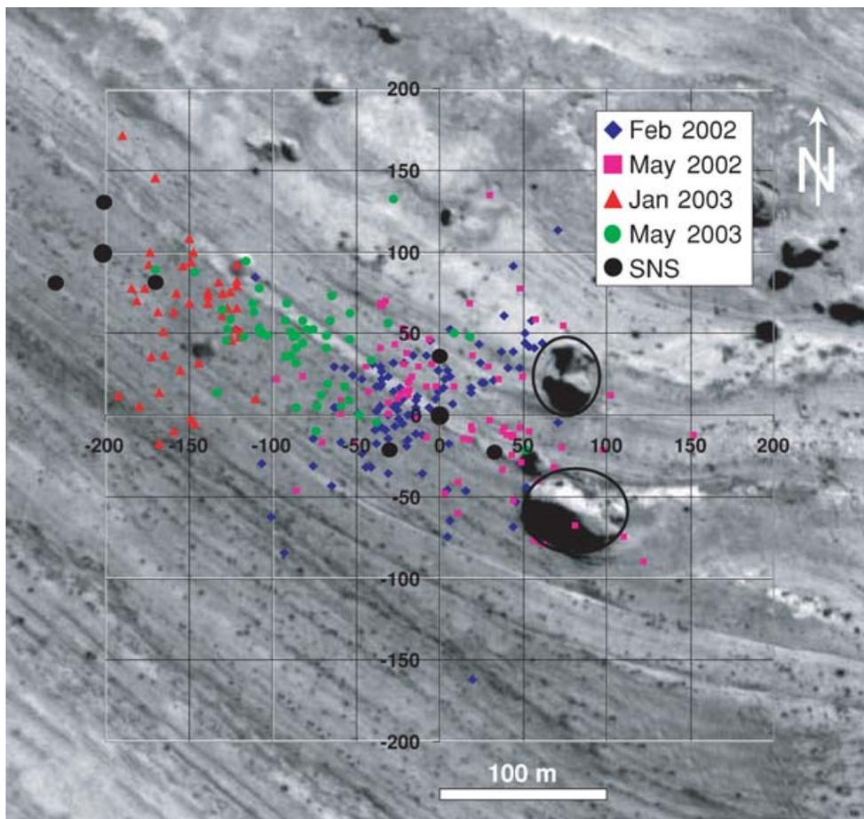
**Figure 9.** Location plot of sinkhole-generated events recorded at Nachal Hever site (Dead Sea) during four 12 hr periods. An air photograph (1999.02.12) of the same location with two fully developed sinkholes (black circles) is provided for comparative purpose. Black circles indicate the location of SNS and its sensors.
