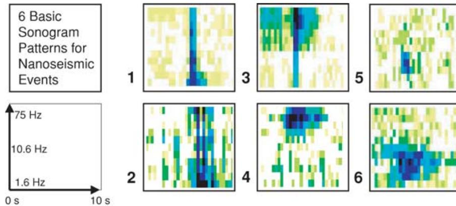
**Figure 3.** Classification of seismic signals by sonogram analysis. Heuristically, six basic signal patterns have been identified and sorted into three subgroups: spikes (#1 and #2), high-frequency events (#3 and #4) and low-frequency events (#5 and #6). For identification of source processes see text.
