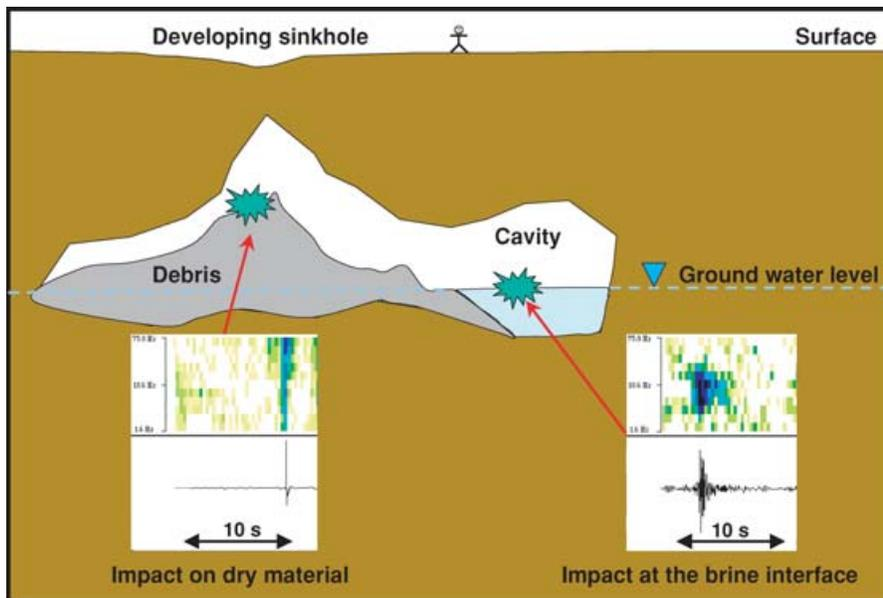
**Figure 12.** Schematic diagram of a sinkhole with two stages of cavitation maturity that are associated with impact type. The sonogram analysis allows the discrimination between dry impacts and impacts in brine-filled cavities, therefore, monitoring pre-collapse sinkhole activity.
