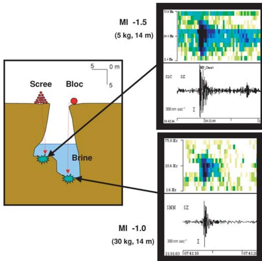
**Figure 7.** Source signal simulation in the field: Waveforms and sonograms generated by impacts in an open brine-filled sinkhole by a rock-debris fall (top) and by a single bloc (bottom).
