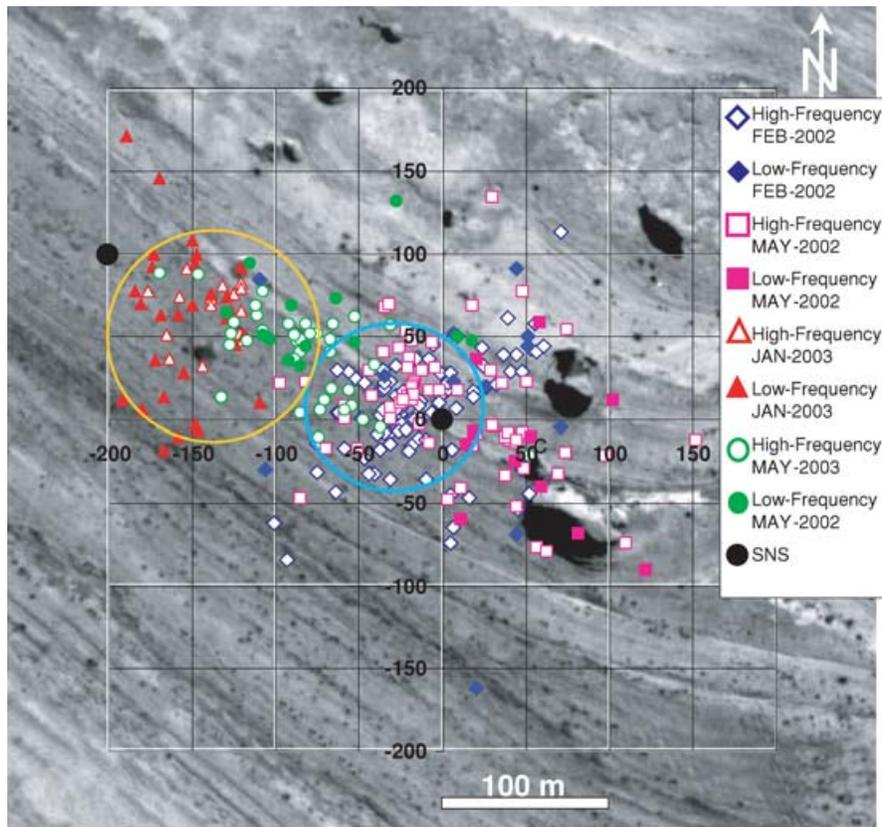
**Figure 11.** Spatial distribution of sinkhole event types recorded at Nachal Hever site (Dead Sea) during four 12 hr periods. Open symbols represent impacts on dry material. Impacts at the brine interface are indicated by filled symbols. The migration of nanoseismic events from the turquoise to the yellow circle denotes an evolution of the sinkhole activity.
